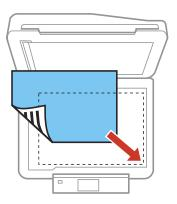
**Note:** You can place multiple originals on the scanner glass. Just make sure they are at least 0.20 inch (5 mm) away from each other and from the edge of the scanner glass.
